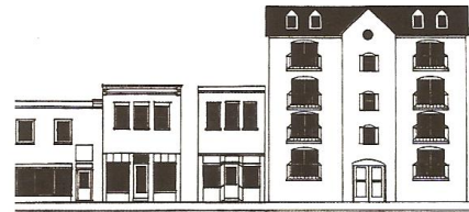
A building that is not appropriate in height, width, or style.
